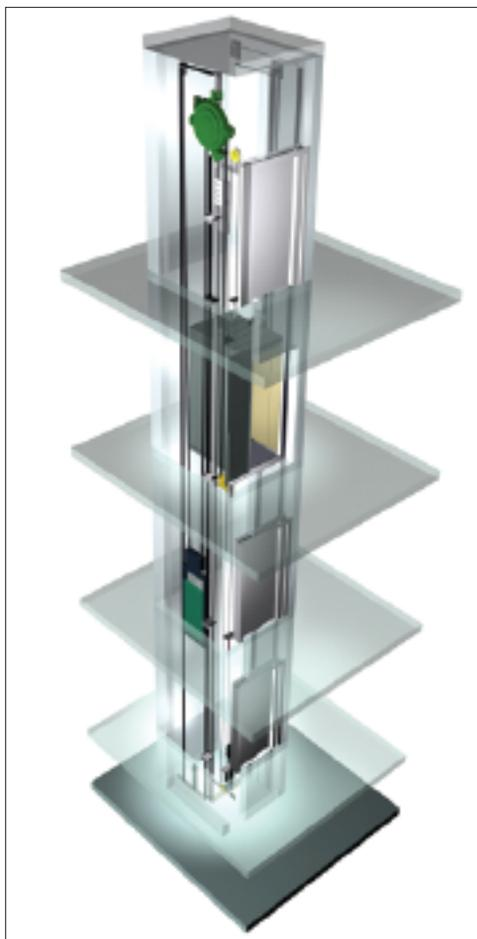
◀ Illustration of a traction elevator
